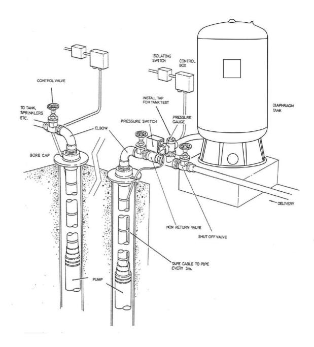
Pump connected for manual operation
